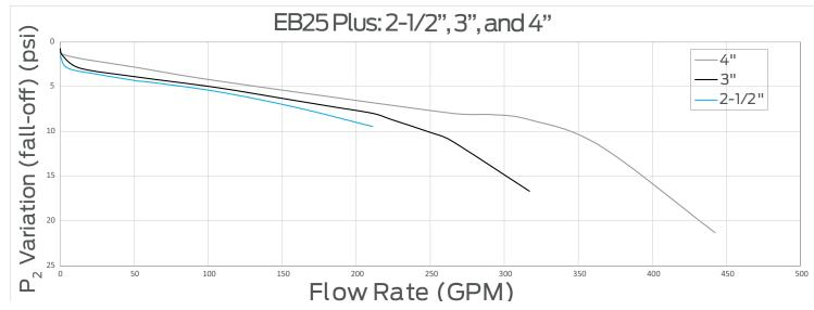
**Pressure Differential:** Difference between the inlet pressure and the PRV set pressure.
