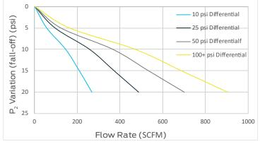
Pressure Differential: Difference between the inlet pressure and the PRV set pressure.
