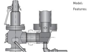
Illustration shows a discharge elbow and drip pan unit attached to a safety valve with female NPT outlet. For safety valves with flanged outlets - 2" to 4" - use companion flange, short nipple and drip pan elbow, all same size as valve outlet. 6" and 8" elbows have integral 125# ANSI B16.1 Flange.
